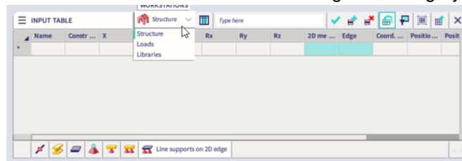
Switching between data in one category is done by clicking on the icons on the bottom of the input table. The icons are the same as in the input panel.
